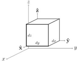
$$\begin{aligned} \operatorname{div} \mathbf{A} &= \lim_{V \rightarrow 0} \frac{\iint_{\partial V} \mathbf{A} \cdot d\mathbf{S}}{\iiint_V dV} = \frac{A_x(x+dx)dydz - A_x(x)dydz + A_y(y+dy)dx dz - A_y(y)dx dz + A_z(z+dz)dx dy - A_z(z)dx dy}{dx dy dz} \\ &= \frac{\partial A_x}{\partial x} + \frac{\partial A_y}{\partial y} + \frac{\partial A_z}{\partial z} \end{aligned}$$
