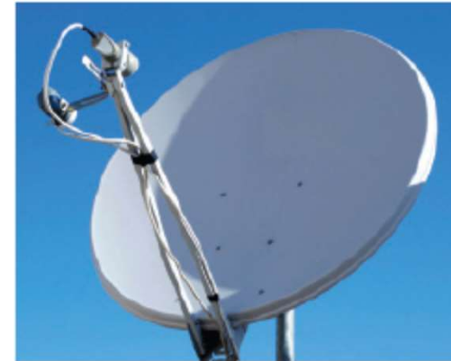
Parabolic surfaces: eliminate spherical aberration
