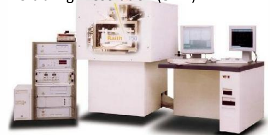
RAITH 150 E-BEAM Ultra high resolution (8nm)
