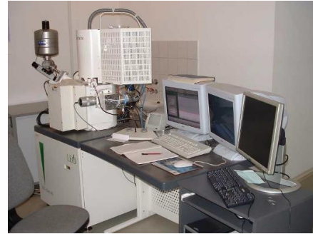
RAITH 150 E-BEAM Ultra high resolution (8nm)
