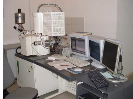
RAITH 150 E-BEAM Ultra high resolution (8nm)
