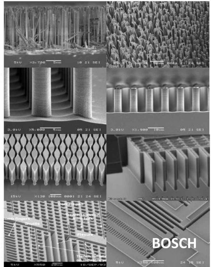
Figure 27. Typical result for room temperature pulsed-mode DRIE (see figure 19).
