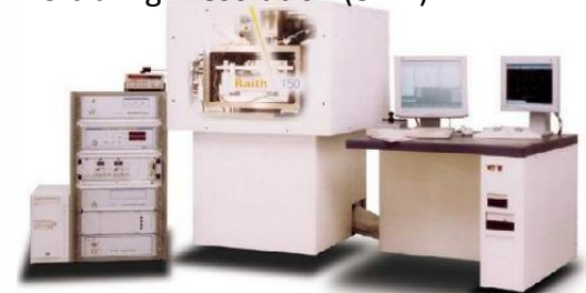
RAITH 150 E-BEAM Ultra high resolution (8nm)
