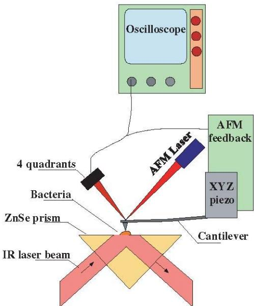
Fig. 1. Experimental setup of the AFMIR.
