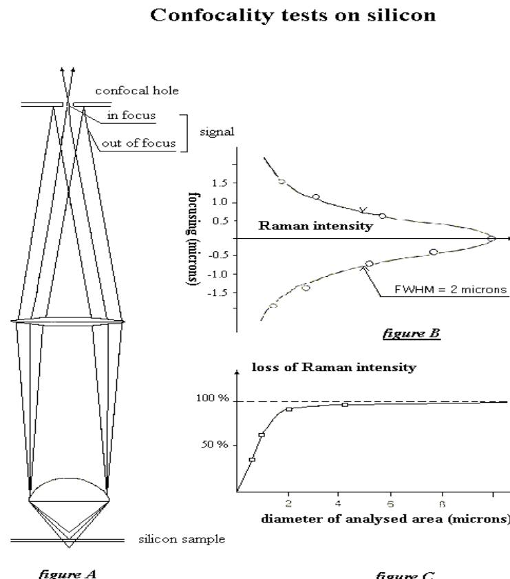
*The confocal pinhole acts as an adjustable spatial filter allowing a precise selection of the analysed volume*
