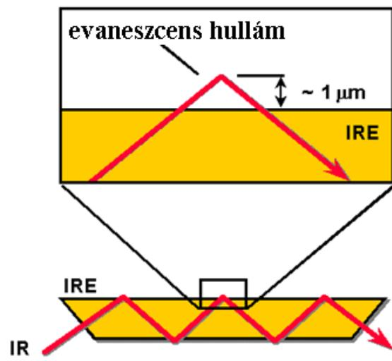
ATR probes a narrow layer close to the surface – solvents with high absorption give measurable signal
