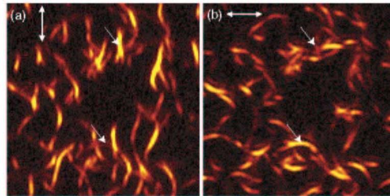
Confocal Raman image of carbon nanotube bundles
