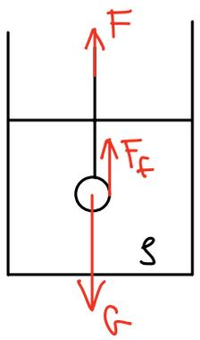
$$\left. \begin{aligned} F_1 + \rho_0 V g &= G \\ F_2 + \rho' V g &= G \end{aligned} \right\} \Rightarrow F_2 + \rho' \cdot \frac{G - F_1}{\rho_0} = G$$
