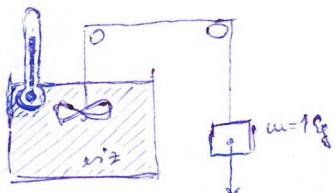
$$\begin{aligned} W_{mech} &= \Delta E_{pot} \approx 10J \\ 1\text{ g wt}, C_{vit} &= 4,2 \frac{\text{J}}{\text{gK}} \end{aligned} \quad \left. \right\} \Delta T = 2\text{ mK}$$
