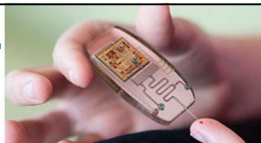
(Top) lab-on-chip (LOC) devices that can be used at the "point of need." (Bottom) Scheme of a silicon based LOC device for Blood testing
