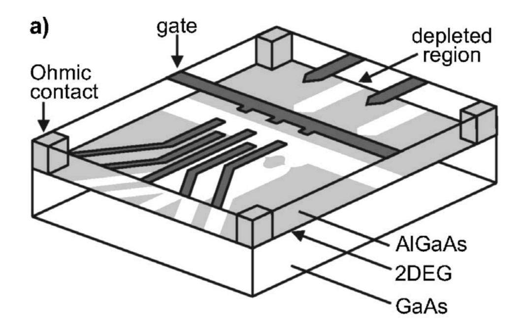
2DEG (2D electron gas) confined in GaAs at the GaAs/AlGaAs interface AlGaAs layer height ~ 30 nm, gate features ~ 50 nm
