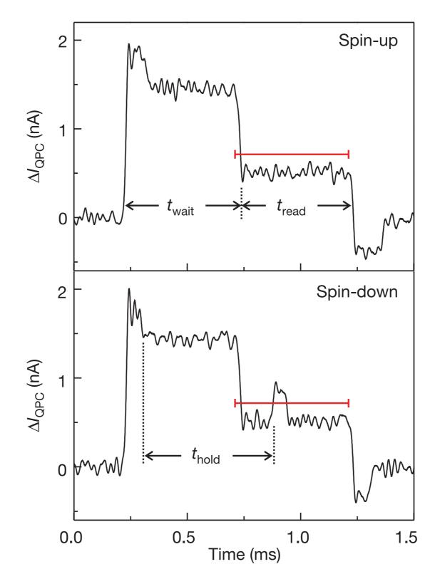
Readout time scale: millisecond. Control time scale (q-gates): microsecond.
