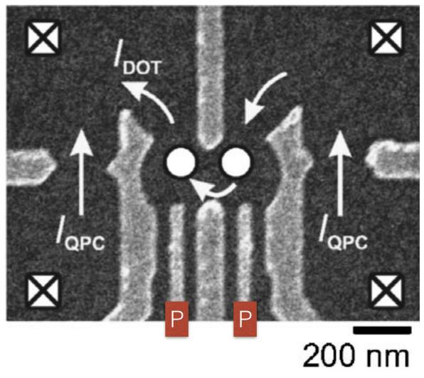
P: Plunger gates: tune (mostly) the on-site potential energy QPC: Quantum Point Contact; used as a charge sensor
