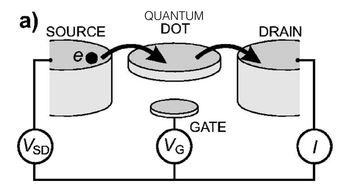
Gate voltage tunes the number of electrons in the quantum dot
