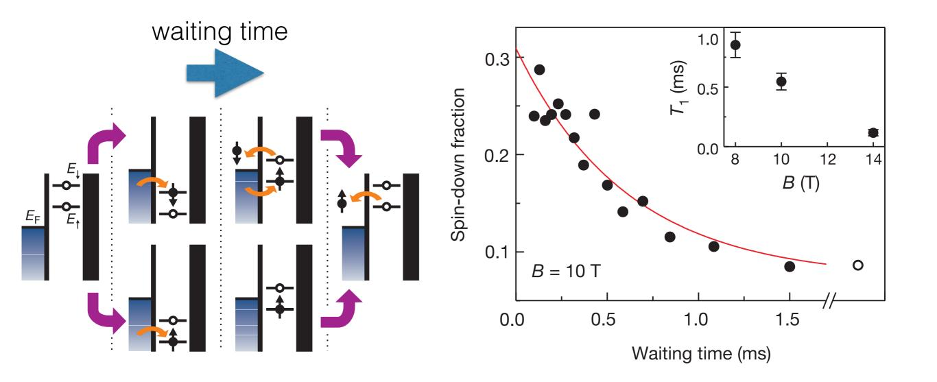
spin relaxation: exponential decay,  $P_{\downarrow}(t_{\text{wait}}) \approx \frac{1}{2}e^{-\frac{t_{\text{wait}}}{T_{\text{spin}}}} = \frac{1}{2}e^{-\Gamma_{\text{spin}}t_{\text{wait}}}$
