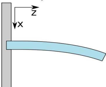
A thin and heavy rod of length  $L$  is horizontally fasten in a wall (see figure). The other end of the rod is free. The axis of the (non bent) rod is the z axis while the vertical axis is the x axis. The Young's modulus of the rods material is  $E$ , the cross-section parameter is  $\Theta$ , and the rod's linear mass density is  $\rho$ .
