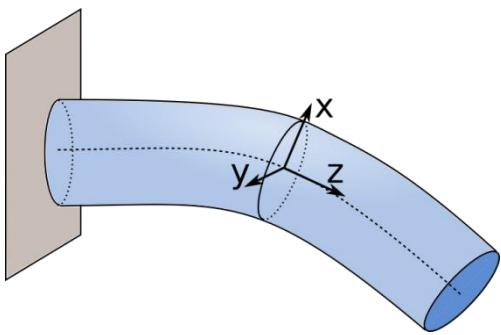
A thin and long elastic rod is bent. In this problem our goal is to describe the stress and deformation tensors in the rod.
