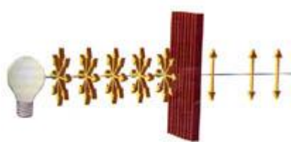
A polarizing filter transforms natural elliptically polarized light to linearly polarized light.
