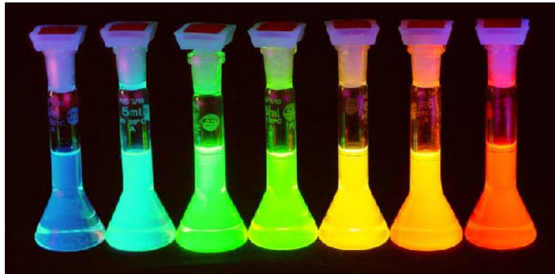
Fluorescence of different sized CdSe quantum dots
