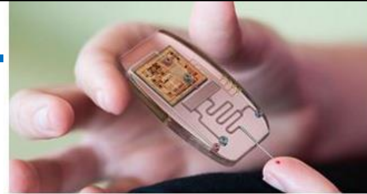
(Top) lab-on-chip (LOC) devices that can be used at the "point of need." (Bottom) Scheme of a silicon based LOC device for Blood testing
